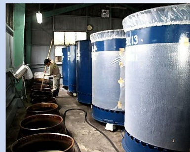
Pots in the first preparation and the enamel cast iron tanks for the second preparation
